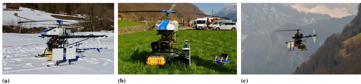
Figure 1: The Gamma L-band SAR mounted on Aeroscout’s UAV Scout B1-100 before take-off (a) in Feb. and (b) in Mar. 2019, and (c) during the repeat-pass multi-baseline SAR data acquisition in Wolfenschiessen, Switzerland, in March 2019. The compact radar hardware and the instrument computer are enclosed in the yellow pelicase. The two quadratic patch antennas (transmit and receive antennas) are mounted close to the Honeywell HGuide n580 INS/GNSS navigation system.
