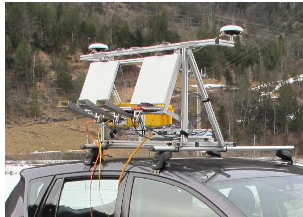
Figure 1: The dual-frequency car-borne SAR setup with (1) the Gamma L-band SAR [1, 2] system with the two (Tx & Rx) white polarimetric patch antennas and (2) the Ku-band GPRI [4, 5] in SAR mode with Horn antennas. The two radar systems can be operated simultaneously. A Honeywell HGuide n580 INS/GNSS system with a local GNSS reference station are used for positioning.
