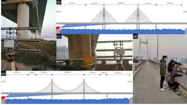
Fig. 3. (a) and (c) In situ measurement setup. (d) GPS receiver being installed on the bridge balustrade. (b) and (c) Sketches of the Yinpenling Bridge and Sanchaji Bridge, respectively.
