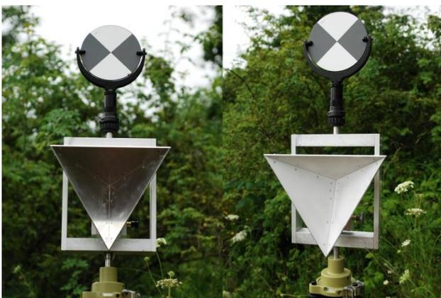
Figure 5: Target without (left) and with dulling spray (right)
