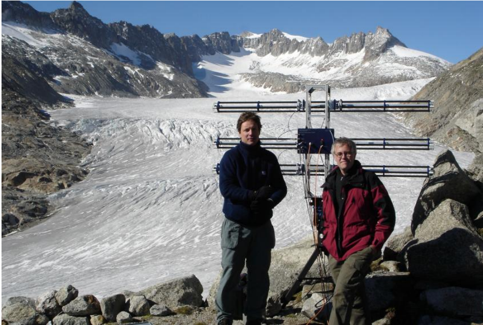
Figure 4: GAMMA terrestrial radar interferometer in Front of the Rhone glacier.
