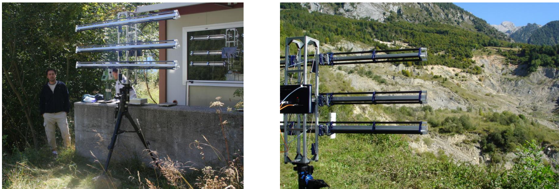
Figure 1 left: GAMMA terrestrial radar interferometer. Right: Target area.
