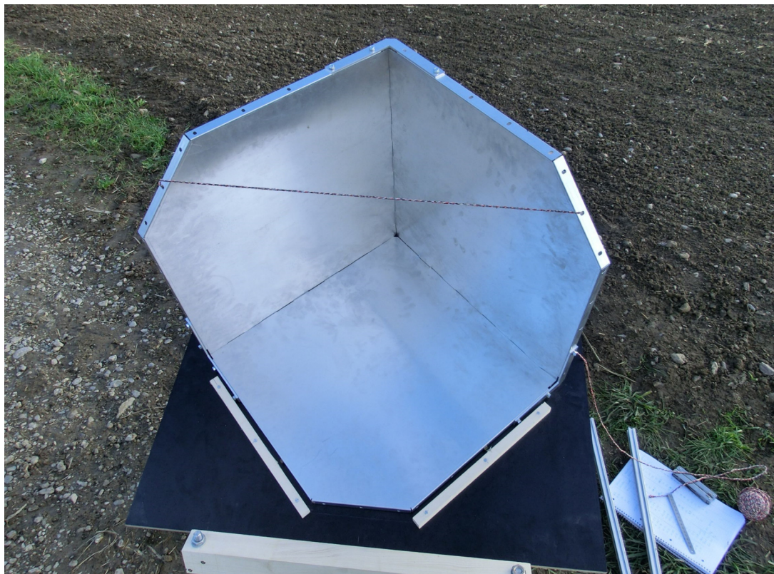
Figure A.21: Symmetrical deformation with the chord spanned from one angled reflector edge to the other
