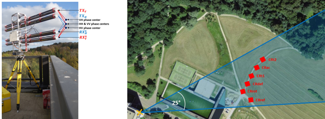
Figure 2.1: Left picture: Setup of the KAPRI radar. The upper 2 antennas (TX) are transmitting while the lower two (RX) are the receiving antennas (Photo: Silvan Leinss) right picture: Overview of the experiment setup on campus ETH Hönggerberg [10]. The position of the Kapri radar is illustrated through the yellow x on the lower left corner. The blue triangle marks the scanned area and the red squares indicate the position of the corner reflectors
