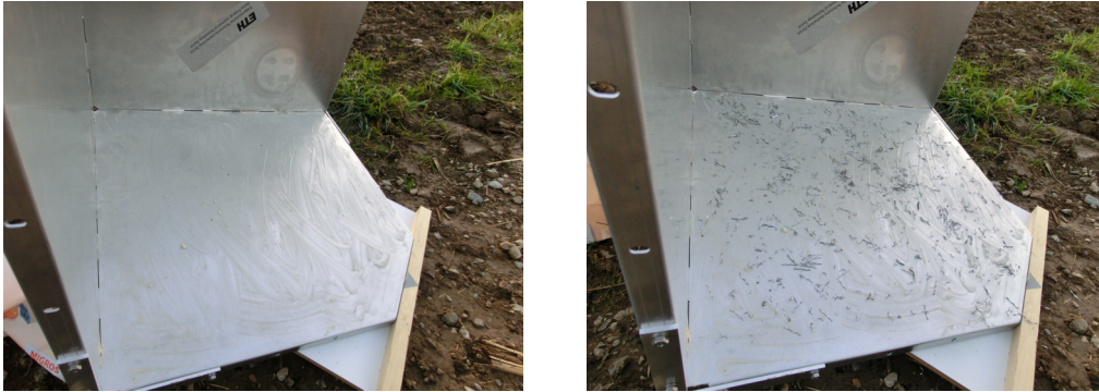
Figure A.18: Aluminum chipping in the reflector according to the measurement protocol A.2 for thin film of paste (left photo) and aluminum chipping (right photo)
