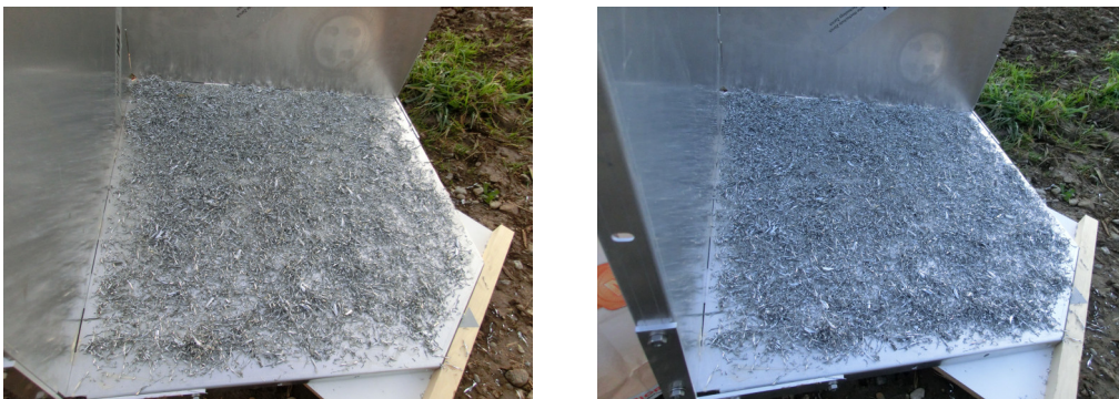
Figure A.20: Aluminum chipping in the reflector according to the measurement protocol A.2 for a lot aluminum chipping (left photo) and all aluminum chipping (right photo)
