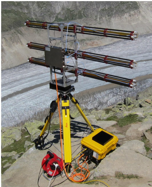
Figure 1: GPRI Instrument looking down on the Aletsch Glacier on 27-Jun-2011.
