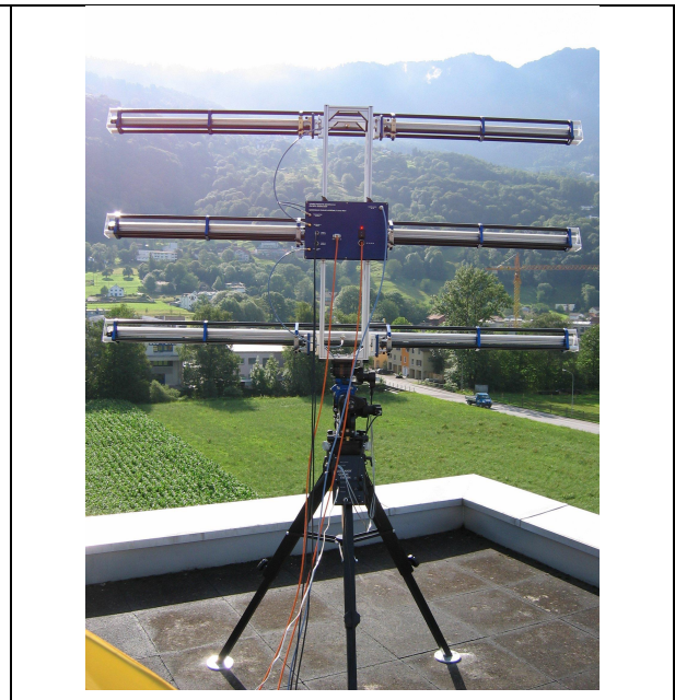
Figure 2. Deployed radar interferometer showing the rotational scanner, antenna support structure, antennas, and microwave assembly.
