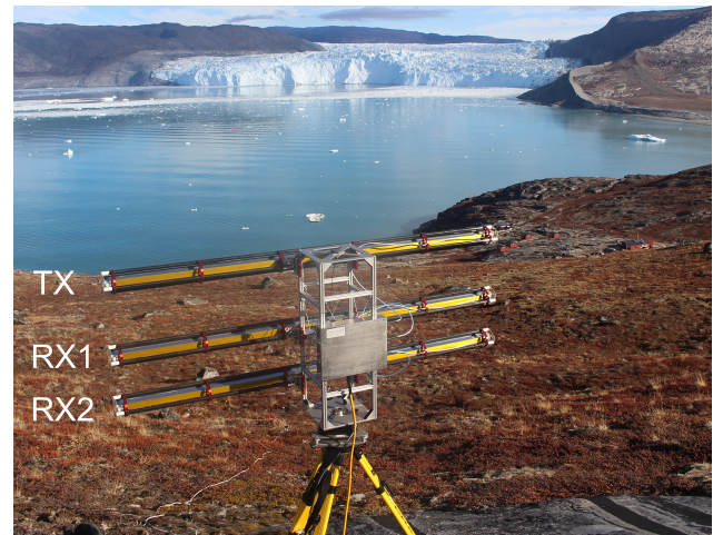
Figure 2. The terrestrial radar interferometer (TRI) located opposite of the front of Eqip Sermia at a distance of 4.5 km (image: M. Lüthi, 2016). The TRI has one transmitting (TX) and two receiving antennae (RX1, RX2).
