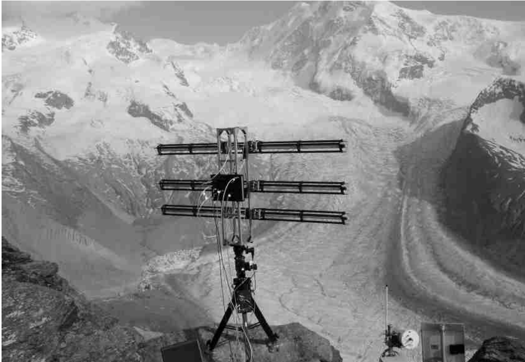
Figure 1. The portable radar interferometer deployed over the Gornergletscher showing the rotational scanner, antenna support structure, antennas, and microwave assembly.
