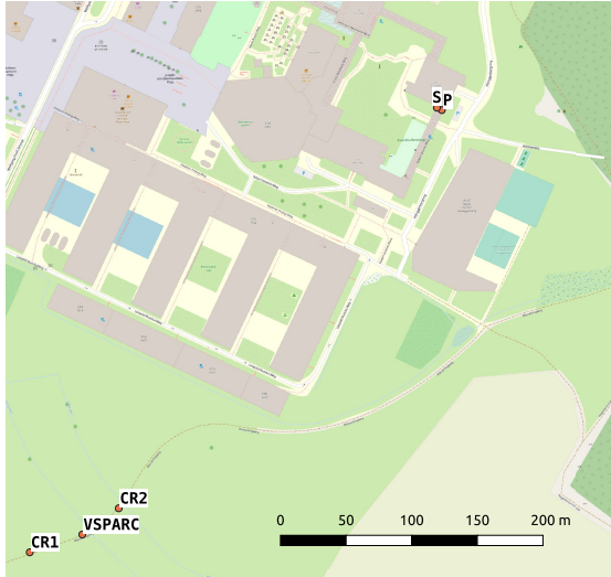
Fig. 14. Polarimetric calibration experimental setup. The primary (P) and secondary (S) devices are placed \sim 1.5 m next to each other and thus are both operating with effectively zero bistatic angle. The calibration targets CR1, CR2, and VSPARC are all placed at range distance \sim 400 m (however, at different range and azimuth coordinates). This allows the application of both CR and VSPARC calibration methods for both devices and their comparative validation. Map data © openstreetmap.org contributors.
