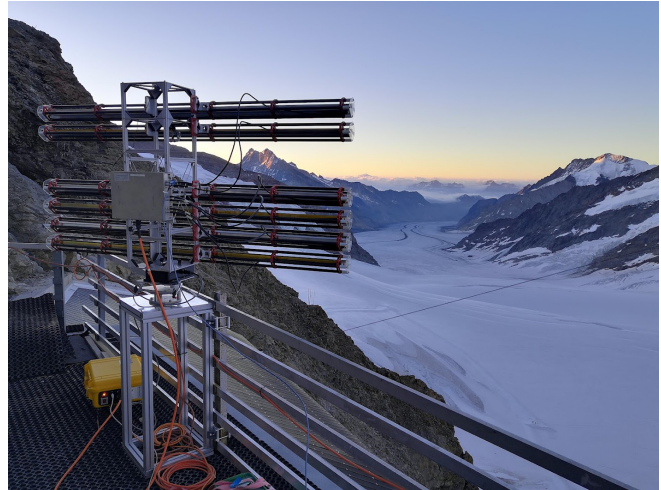
Fig. 1. The primary KAPRI instrument (P) placed on the terrace of the High Altitude Research Station Jungfraujoch, observing the Jungfraufirn area. The rotating tower performs azimuthal sweeps of the scene, acquiring a monostatic, full-polarimetric, single-pass interferometric dataset during each acquisition.
