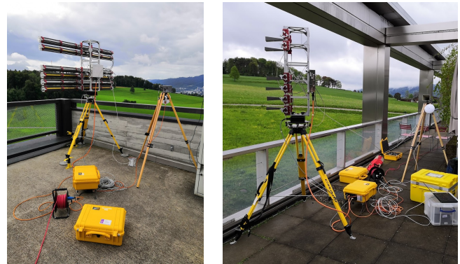
Fig. 1: Bistatic KAPRI device configuration (left: primary device (P) equipped with narrow-beam traveling wave antennas, right: secondary receiver device (S) equipped with horn antennas). Reference link horn antennas are placed on tripods on the right side of the two images, together with long-range Wi-Fi antennas for remote device control.
