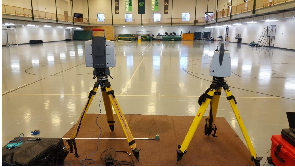
Figure 5.11. From left to right: Leica Scan Station II and Leica Scan Station P40.
