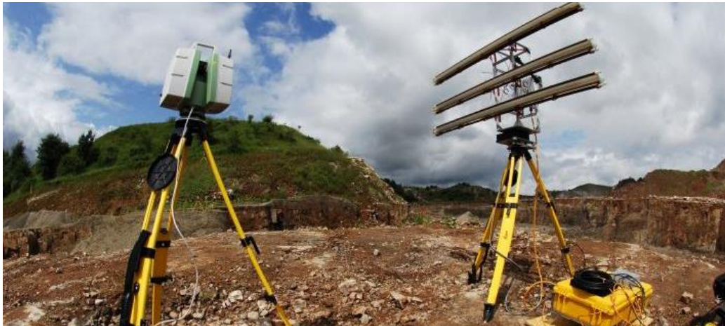
Figure 2.7. To the left is the TLS and to the right is the TRI used by Wujanz et al. (2013).
