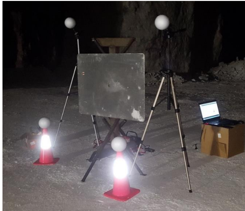
Figure 5.7. Tall steel frame with the linear motion actuator and 106 x 76 cm target.
