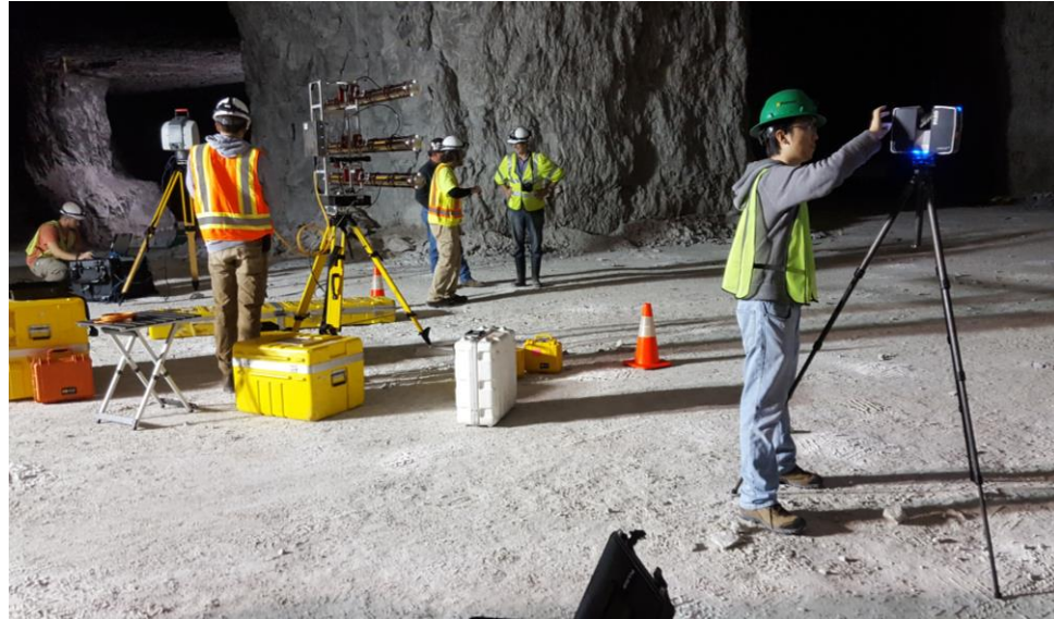
Figure 5.19. Equipment used in Springfield Underground. Missouri S&T Leica Scan Station 2 (to the left), the MU GPIR (center), and the Missouri S&T Faro Focus 3d X130 (to the right).
