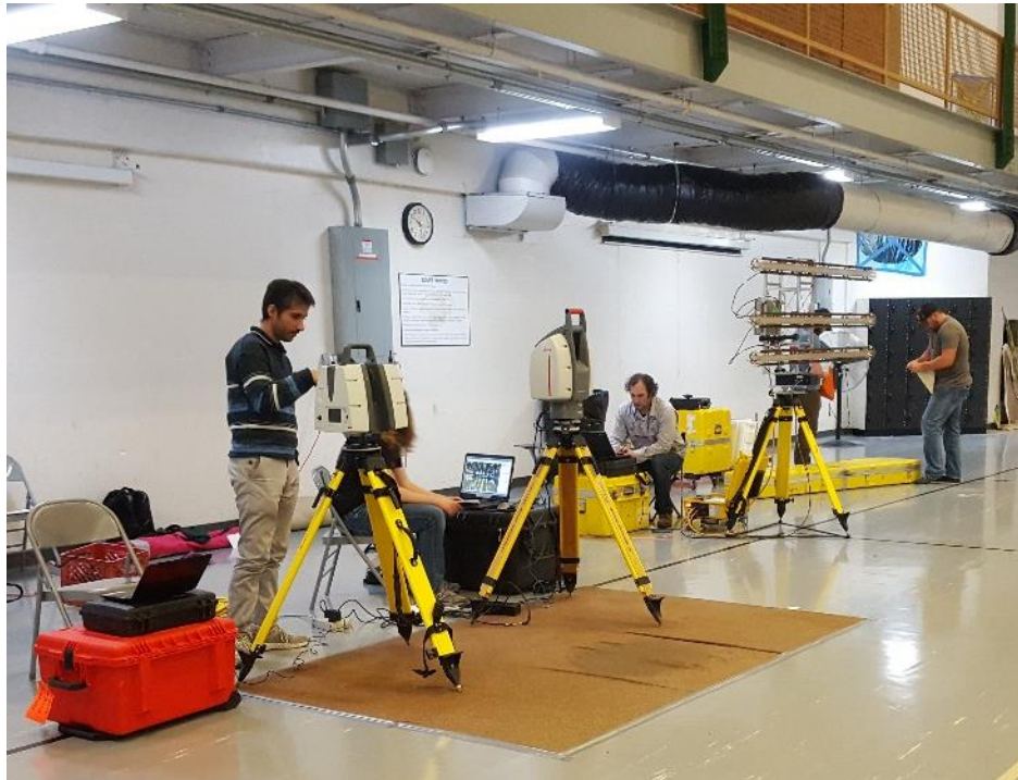
Figure 5.22. Equipment used in the third measurement campaign. From left to right: Leica Scan Station P40, Leica Scan Station II, and Gamma GPIR II.
