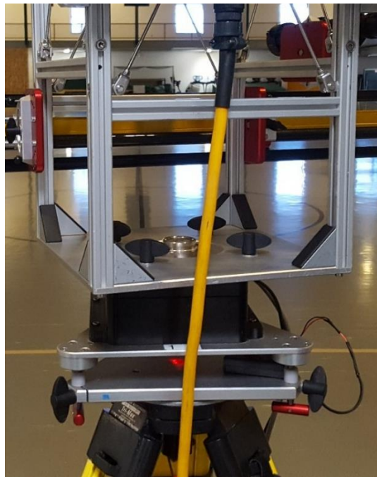
Figure 5.24. The blue dot on rear of the tribrach marks the position from where repositioning displacements were taken.
