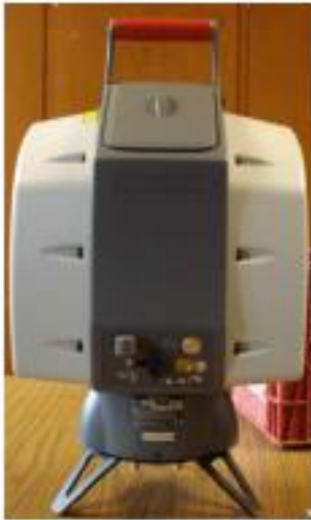
Figure 4.7. A back view for the Leica-ScanStation2 which was used in this research (Aqueel, 2012).
