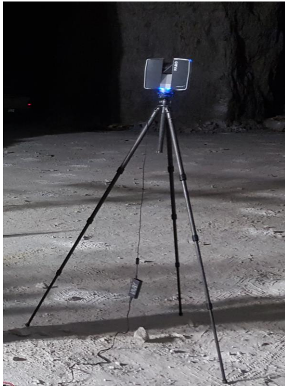
Figure 5.10. Back view of the Faro Focus 3D X130 that was used in the first measurement campaign.
