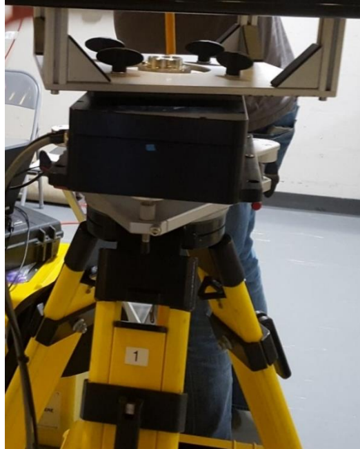
Figure 5.23. The blue dot on front of the azimuthal scanner of the TRI marks the position from where the RDS displacements were taken.
