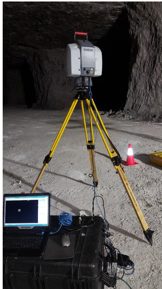
Figure 5.9. A back view of the Leica-ScanStation2 that was used in this research.
