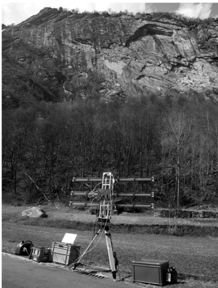
Figure 3 Set-up of the GPRI-I at Soazza using a survey tripod, levelled and centred with respect to a fixed point.
