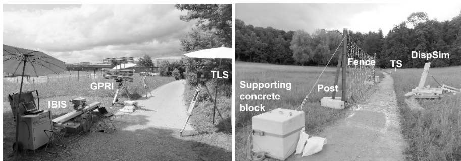
Fig. 2 Sensors used during the experiment: a synthetic aperture IBIS FM radar mounted on two concrete blocks, a real aperture GPRI radar mounted on a tripod, and a TLS placed on a tripod (left). Displacement simulator located behind the fence in the second geometrical configuration (ROCCO fence mounted on steel posts); a total station used for ground-truth measurements is visible in the background (right).
