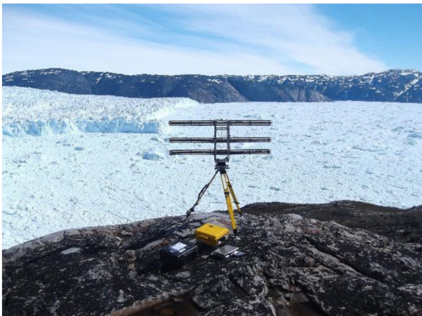
Figure 2. Photo showing set-up of the TRI overlooking the calving front of Store. TRI, terrestrial radar interferometer.
