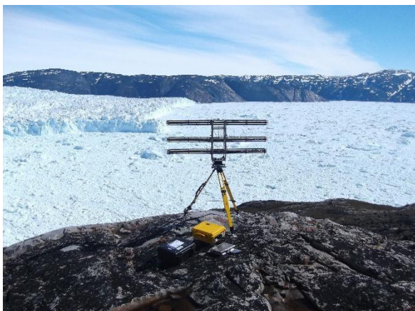
Figure 4 – Set-up of the TRI overlooking the calving front of Store.
