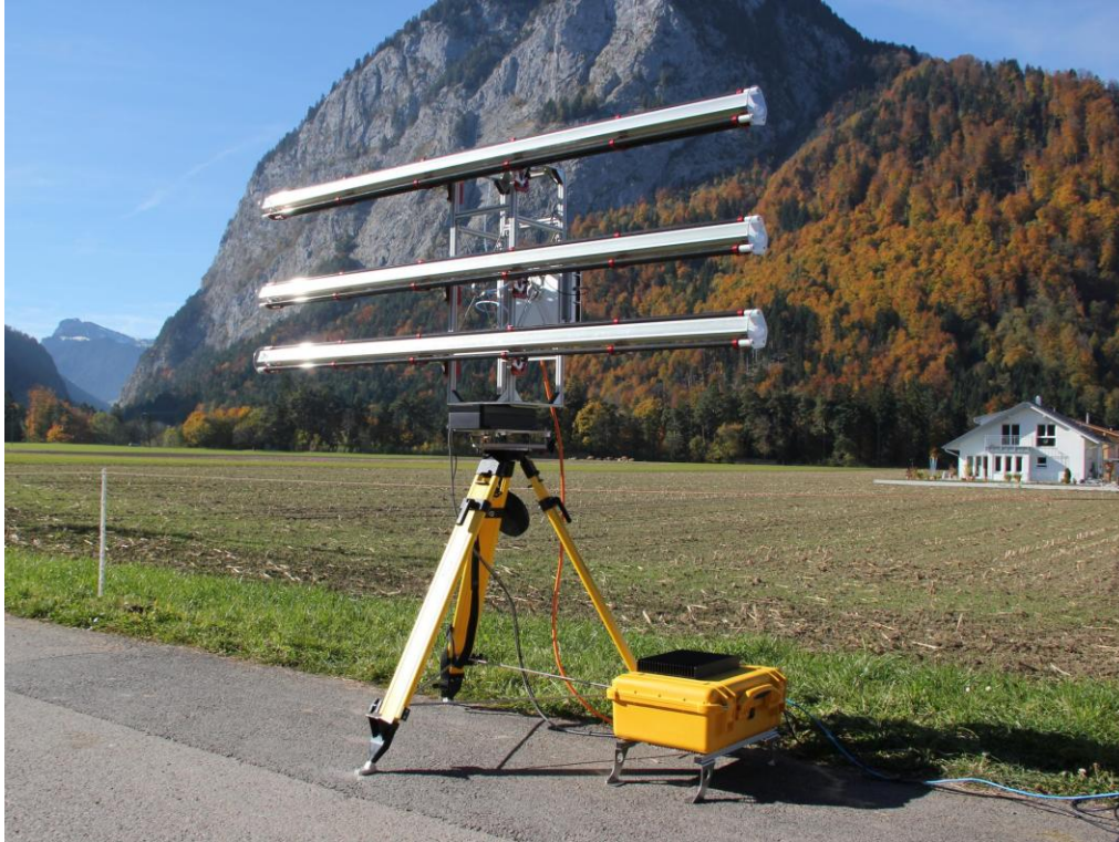
Figure 2.5. GPRI-II acquiring images of a mountain near Gumligen, Switzerland on October 31, 2010 (from GAMMA Remote Sensing AG, 2011).
