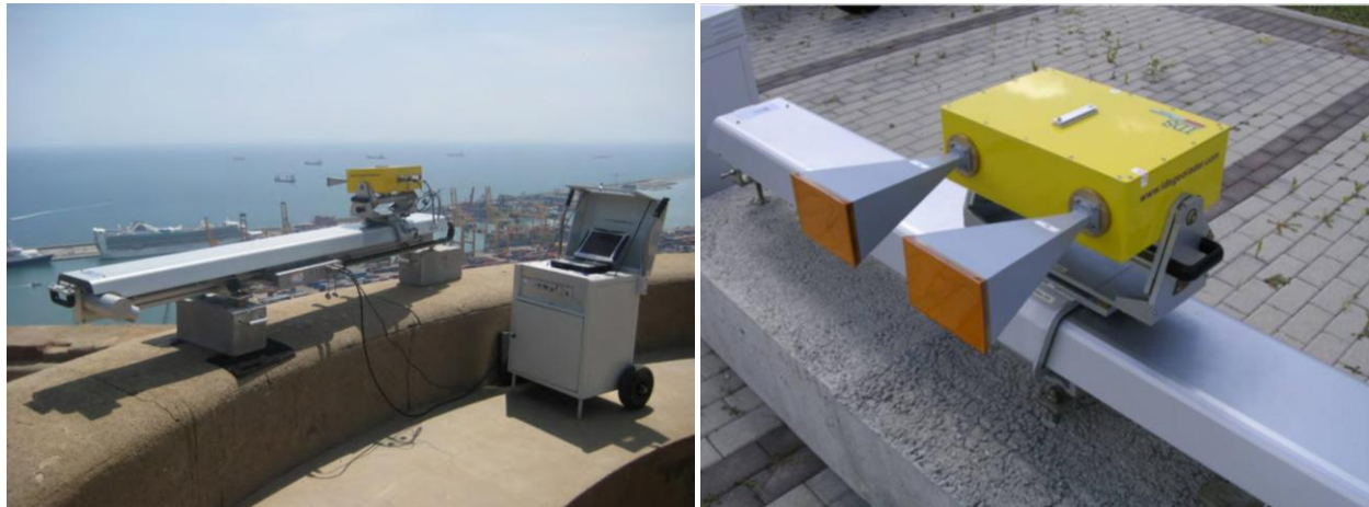
Figure 2.8.a) IBIS-L RADAR system: rail, sensor module, and computer/power component (from (Jungner, 2009), b) IBIS-L sensor module composed of receiver and transmitter antennas (from Ingegneria Dei Sistem Website, 2012)
