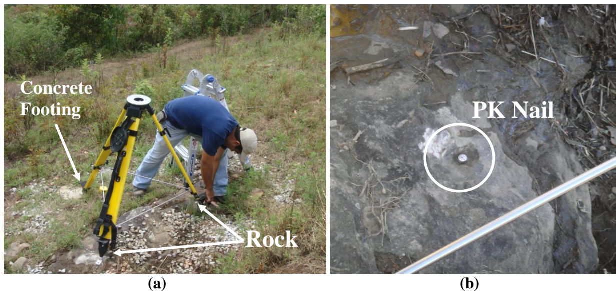
Figure 4.19. a) Anchoring tripod to rock at the Overlook viewpoint, and b) PK nail in rock used to center the GPRI-II at the Overlook viewpoint near Chester, Arkansas.
