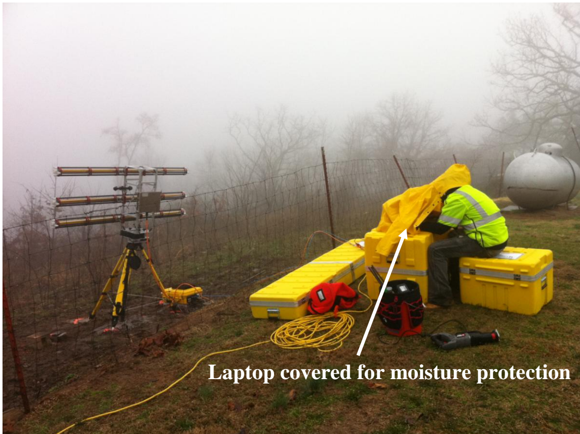
Figure 4.24. GPRI-II acquiring data during fog in overlook viewpoint (calibration site) near Chester, Arkansas.
