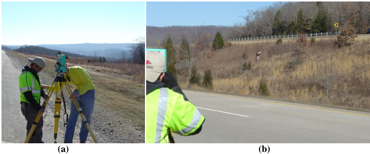
Figure 3.10. Researchers from the UofA a) preparing the total station for data acquisition, and b) acquiring topographic data at the calibration site near Chester, Arkansas.
