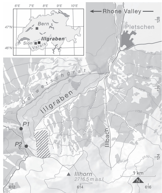
Fig. 1. Location of the Illgraben debris flow catchment showing area of investigation (hatched), position of GPR for various campaigns (labeled P1 and P2), and forested areas (shaded gray).
