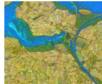
RGB composite of ERS coherence (red), average backscatter (green), and backscatter temporal variability (blue) over the Netherlands.
