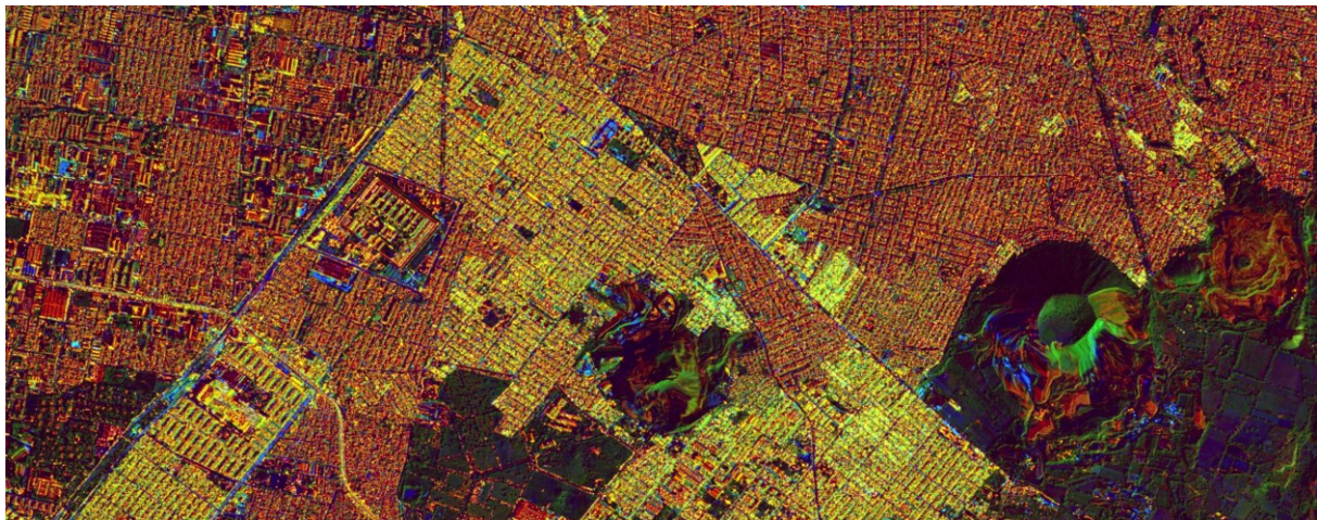
Figure 12 RGB composite of average coherence, average backscatter and backscatter temporal variability calculated for the Capella X-band stack over Mexico City. The top image shows the complete area covered by the stripmap acquisitions; the bottom image is a more detailed view on a smaller section. The arrow indicates the radar look direction (at 40.5 deg. incidence angle). Yellow areas correspond primarily to buildings with very high backscatter from structures oriented perpendicular to the look direction.
