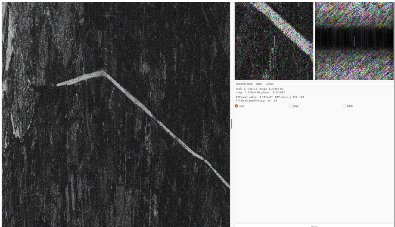
Figure 1 SLC spectrum of the SWOT data. In the azimuth direction the spectrum is not centered due to a significantly non-zero Doppler Centroid. In the range direction, the spectrum does not seem to be clearly constrained, possibly related to the time-domain back-projection processing used to focus the data.
