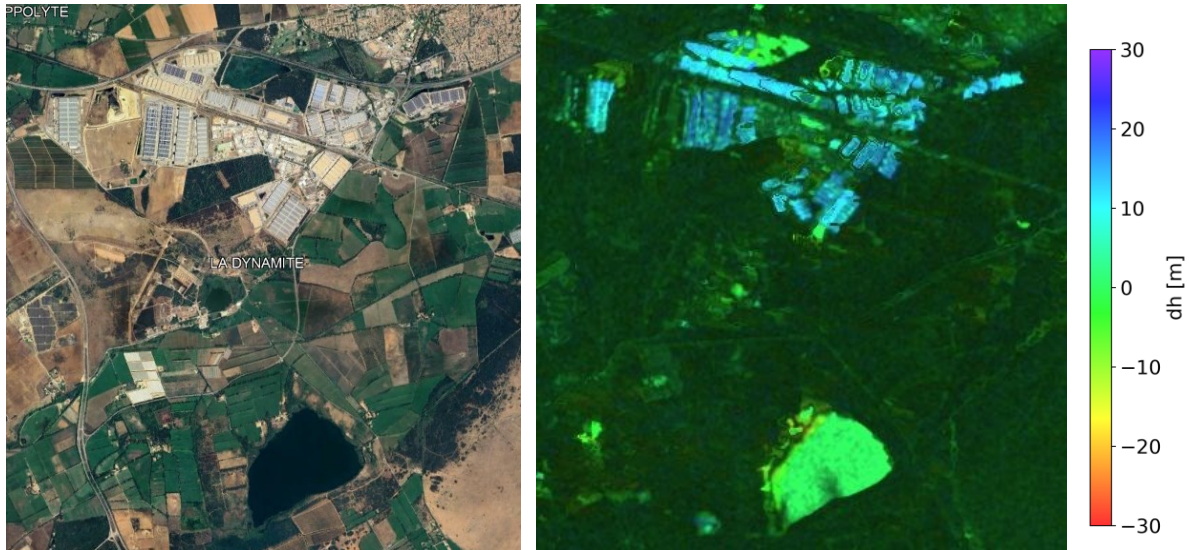
Figure 9 Positive height corrections are observed for new industrial buildings in the Camargue, France. The height of these buildings is not present in the SRTM based height reference used in the SWOT data focusing.
