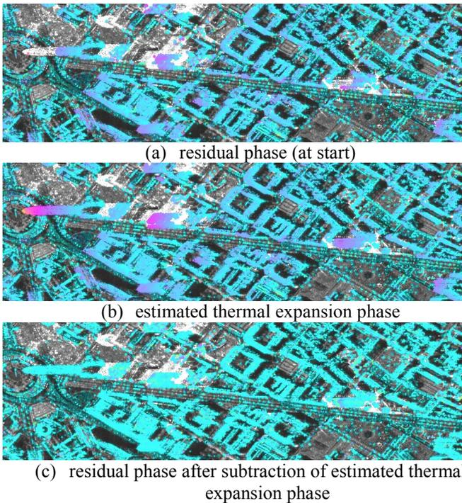
Fig. 2. Example of improvement for one interferometric pair of a TX data stack over a section of Barcelona. One color cycle corresponds to two phase cycles.
