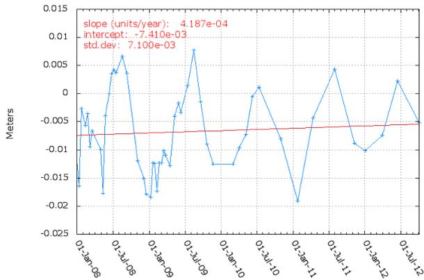
Fig. 6. Deformation time series of a point near the top of the tallest building in Fig. 3.
