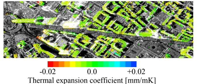
Fig. 7. Thermal expansion coefficient estimate derived from the PSI result.
