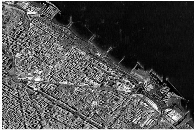
Fig. 1. Averaged backscatter intensity obtained from an interferometric stack of 50 TerraSAR-X data sets showing parts of the city of Barcelona.
