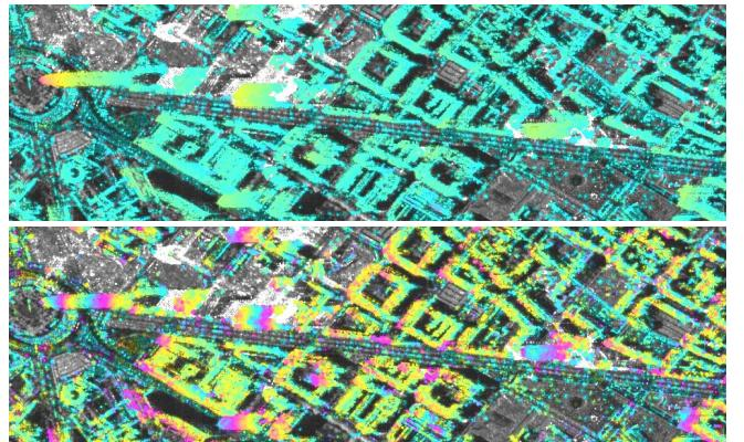
Fig. 3.  $\partial\theta/\partial\text{temp}$  determined for the TX stack over Barcelona, shown using two different color scales: 1 rad/1 deg C per color cycle (top) and 0.2 rad/1 deg C per color cycle (bottom).
