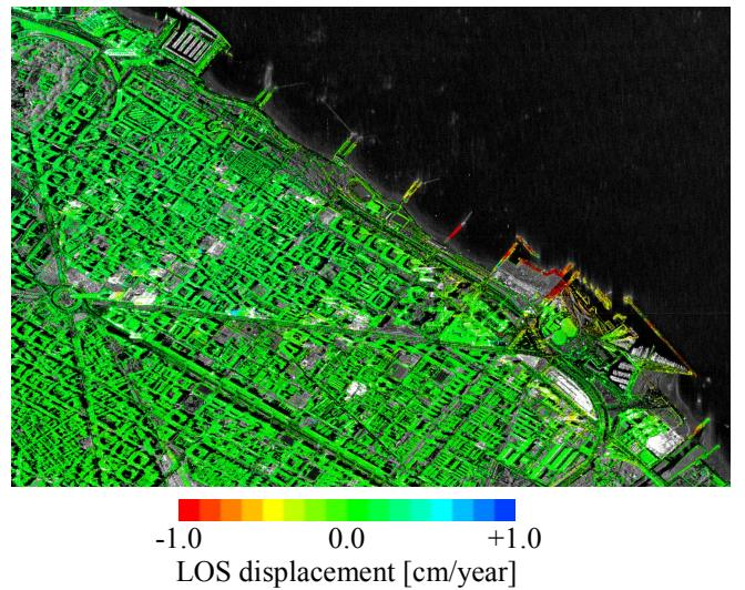
Fig. 5. Average deformation rate estimated from TX stack over Barcelona after mitigation of thermal expansion effects.
