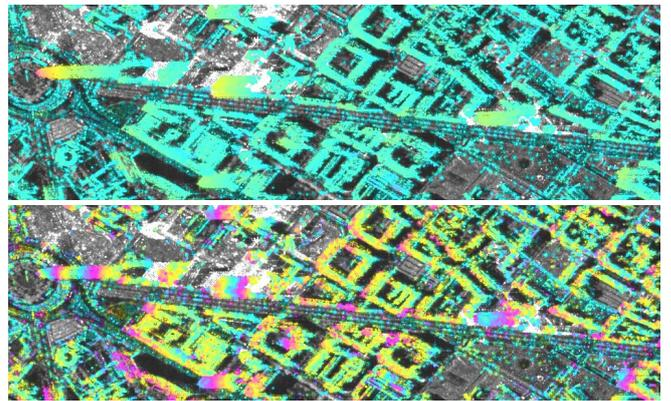
Fig. 3.  $\partial\theta/\partial temp$  determined for the TX stack over Barcelona, shown using two different color scales: 1rad/1deg C per color cycle (top) and 0.2rad/1deg C per color cycle (bottom).
