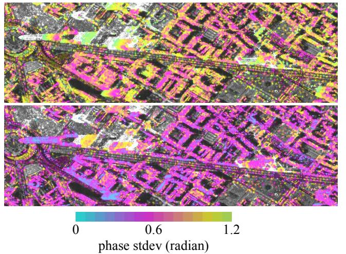
Fig. 4. Phase standard deviation from bi-linear linear regression without (top) and with (bottom) subtraction of the thermal expansion phase.
