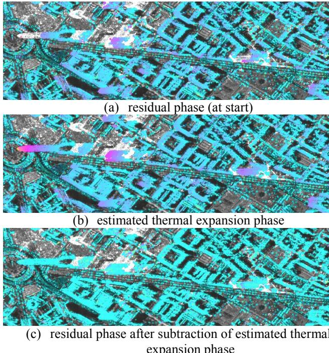
Fig. 2. Example of improvement for one interferometric pair of a TX data stack over a section of Barcelona. One color cycle corresponds to two phase cycles.
