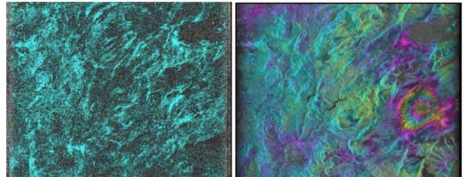
Figure 2 Aquila Earthquake, Italy. For the PALSAR pair 20080720 – 20090422 the split-beam interferogram (left) clearly indicates that the co-seismic interferometric phase (right) is not much affected by an ionospheric path delay. In both images one color cycle corresponds to one phase cycle. Image shown is in slant range geometry and corresponds to a full frame.
