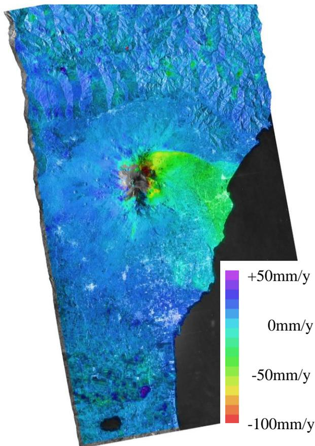
Figure 5 Linear deformation rate derived using 19 PALSAR scenes between 20070127 and 20100322.
