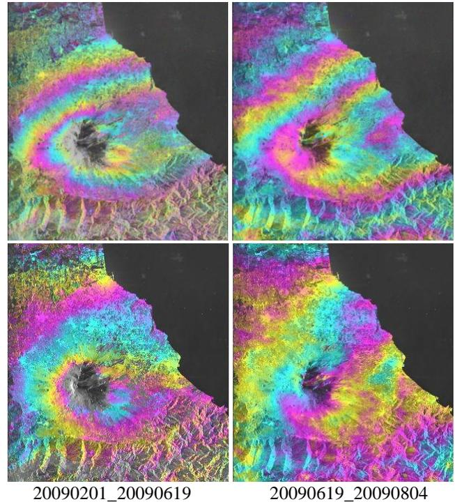
Figure 4 Two PALSAR differential interferograms (top) including the scene on 19-Jun-2009 over the Etna and corresponding "ionospheric delay corrected" interferograms (bottom). A color cycle corresponds to a phase cycle.
