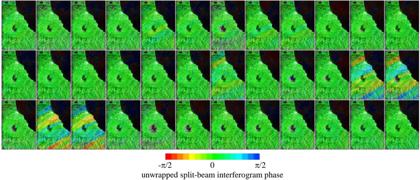
Figure 3 Multi-reference stack of PALSAR split-beam interferograms over the Etna volcano, Italy. The pairs shown are listed in Table 1. Very strong phase variations (ionospheric effects) are observed for the pairs 23,24,26,27 which all include the scene acquired on 19-Jun-2009. The images are shown in slant-range geometry.
