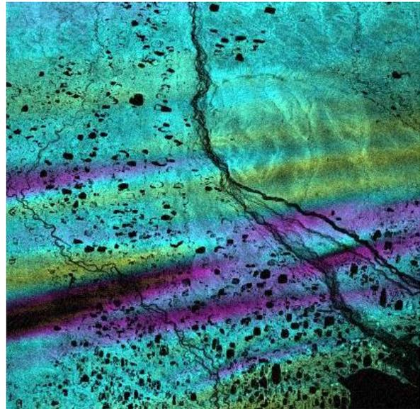
Figure 1 PALSAR multi-look split-beam interferogram of an area in Alaska. One color cycle corresponds to one  $2\pi$  phase cycle. Image shown is in slant range geometry and corresponds to a full frame.
