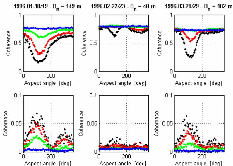
Figure 1. Coherence as a function of aspect angle for the Liaoning image frame (above) and difference between coherence obtained with and without slope-adaptive range common-band filtering (below). Results are showed for four different slope angles (blue = 0°, green = 5°, red = 10°, black = 15°).
