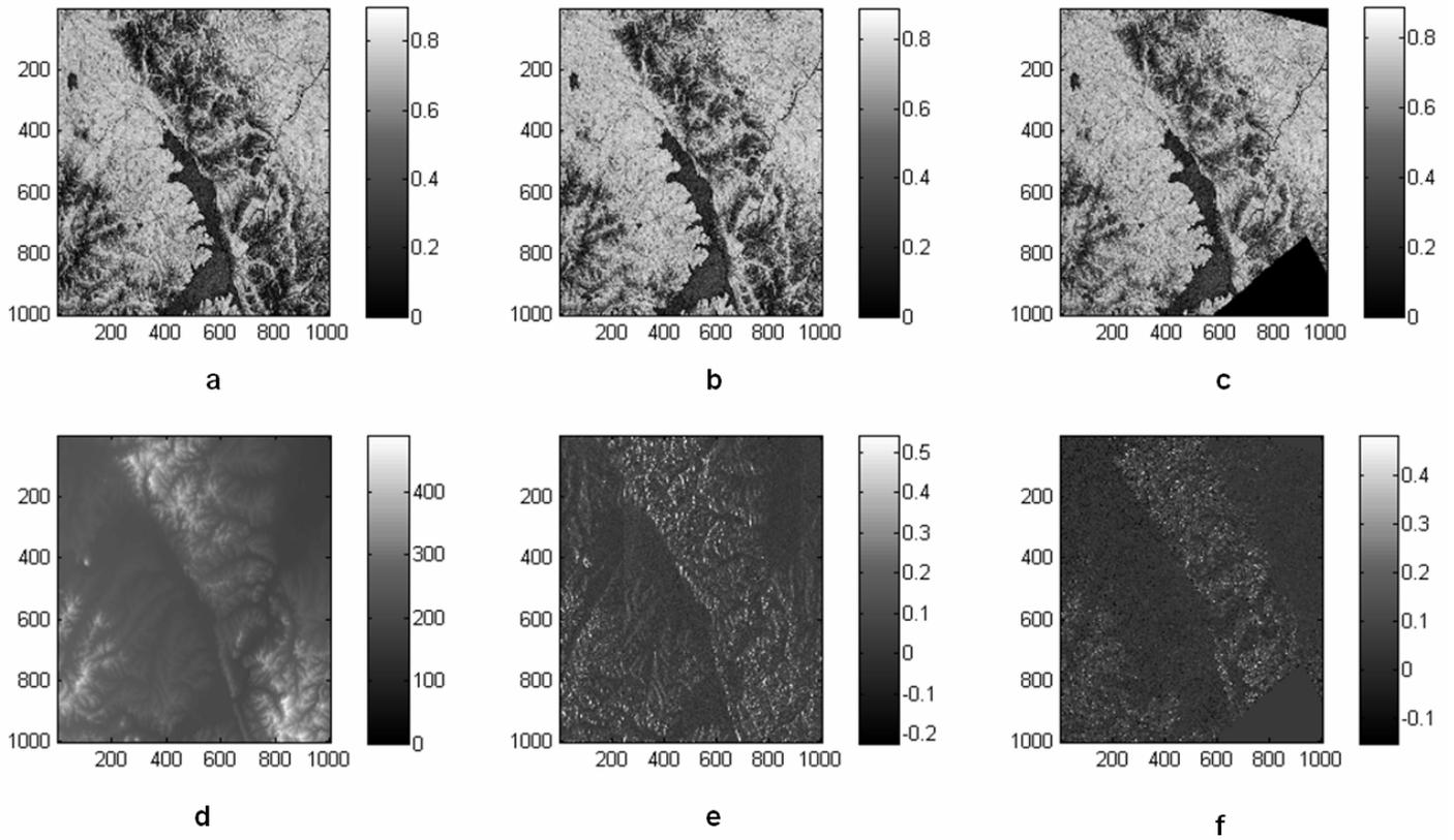
Figure 2. Coherence images obtained without and with slope-adaptive range common-band filtering based on SRTM-3 (a and b), and with slope-adaptive common-band filtering based on SRTM-1 DEM (c). SRTM-3 DEM (d), image difference b-a (e), image difference c-b (f).
