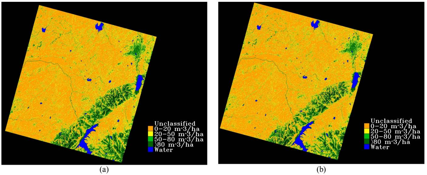
Figure 3. Classified forest stem volume in  $m^3/ha$  using coherence (a) without and (b) with slope-adaptive range common-band filtering. In (b) forested regions have lower biomass or are classified as bare ground (instead of forest) because of the increased coherence after slope-adaptive range common-band filtering.
