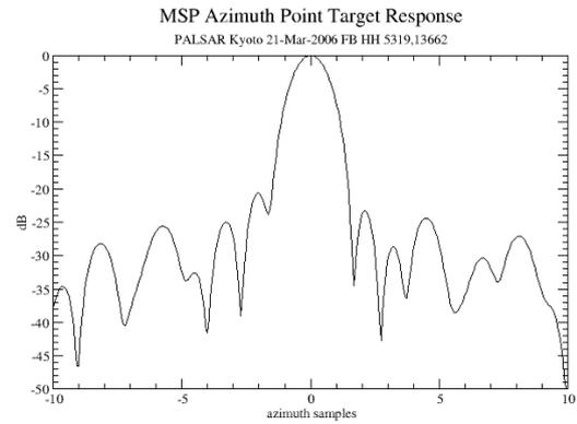
Figure 5. Point target response in azimuth.
