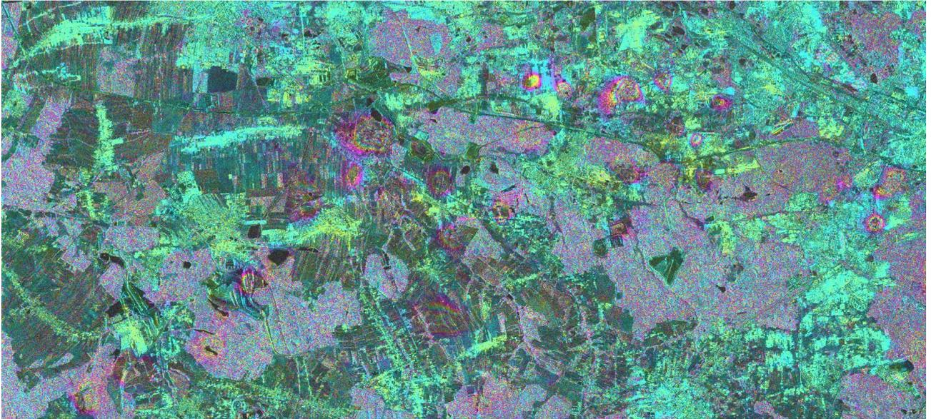
*Figure 5. Section of a georeferenced PALSAR FBS – FBD differential interferogram over mining area in Poland, 20070222\_20070710,  $\Delta t=138$ days,  $B_{\perp}=809$ m. One color cycle corresponds to 11.7cm displacement along the line-of-sight direction.*
