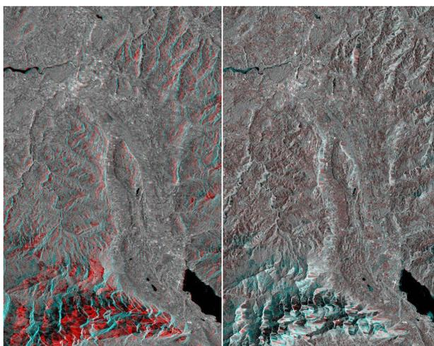
Fig. 2. Region near Bern, Switzerland. In each case, two images have been superposed as red and cyan. For the image on the left a single scene was geocoded first using only an ellipsoid and then including terrain height. Large discrepancies are visible at the bottom of the image. For the image on the right, adjacent ERS swaths (orbits 20918 and 21190) were geocoded using a DEM simulating ASAR data acquired with different look angles.
