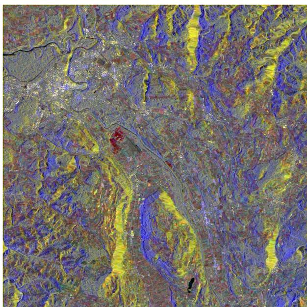
Fig 3. Multi-temporal combination of ascending and descending orbit ERS data for flood mapping. red: descending 21-Apr-1999, green: descending 26-May-1999, blue: ascending: 26-May-1999.
