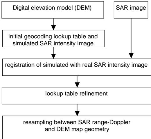
Fig. 1: Flow chart of automated terrain corrected SAR geocoding.
