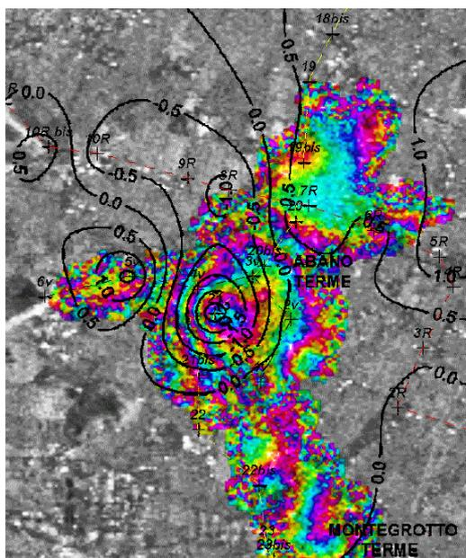
Figure 5. Vertical ground movements (in  $\text{mm/year}$ ) from levelling surveys in 1991 and 1995 in the urban areas of Abano and Montegrotto Terme (data from Comune di Abano Terme and Regione del Veneto) superposed to the interferometric displacement velocity map for the interval 1992 to 1996. Also shown are the position of the levelling lines and benchmarks.
