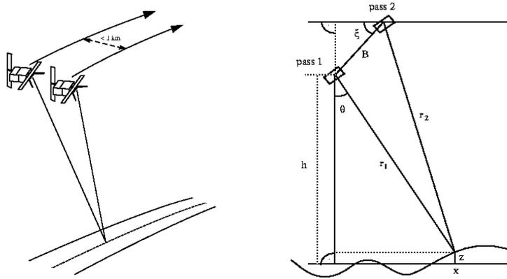
Figure 1: Interferometric imaging geometry showing the two passes with range vectors  $r_1$  and  $r_2$  to the resolution element. The look angle of the radar is  $\theta$ . The baseline  $B$  is tilted at an angle  $\xi$  measured relative to horizontal.
