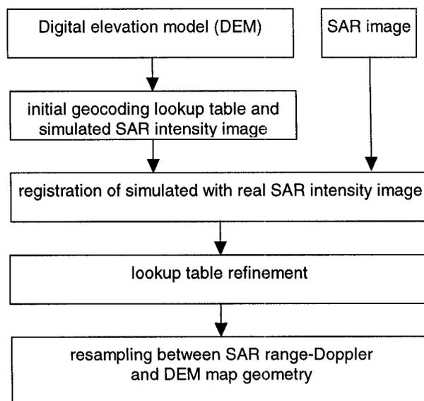
Figure 1: Flow chart of automated terrain corrected SAR geocoding.
