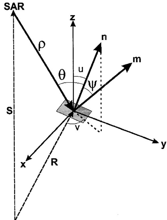
Figure 2: SAR imaging geometry with **vectors**:  $x$  (azimuth),  $z$  (vertical),  $r$  (radar look vector),  $R$  (Earth center to pixel),  $S$  (Earth center to SAR),  $n$  (surface normal), and  $m$  (image plane normal) and **angles**:  $\theta$  (local incidence angle),  $\psi$  (projection angle), and  $u, v$  (spherical angles of  $n$ ).
