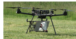
Fig. 2. Gamma L-band SAR (GLSAR) system integrated on a carbon frame, which holds the entire SAR system including the GNSS-aided inertial navigation system (Honeywell HGuide n500), SAR transmit and receive antennas, and two helix-type GNSS antennas. The entire system can be easily attached and detached to/from a vibration-decoupled central mount point of the FreeFly Alta-X UAV or a similar UAV.
