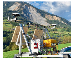
Fig. 1. Gamma S-band SAR system (GSSAR) with a more compact and lightweight form factor (aluminum enclosure with red heat sink) mounted on a car rack for first repeat-pass interferometry demonstration using the S-band system with 400MHz bandwidth at the landslide of Brinzauls in Switzerland. The rack also holds the previous version of the Gamma L-band SAR system (yellow pelicase enclosure), which was used to produce interferograms at L-band for comparison.
